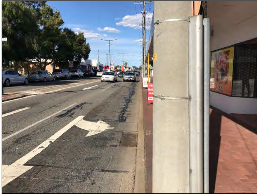
Finding 2.2 – Concrete power pole in a clear zone. Undergrounding power may be a long term goal to remove poles that can't be relocated or protected by a barrier.
